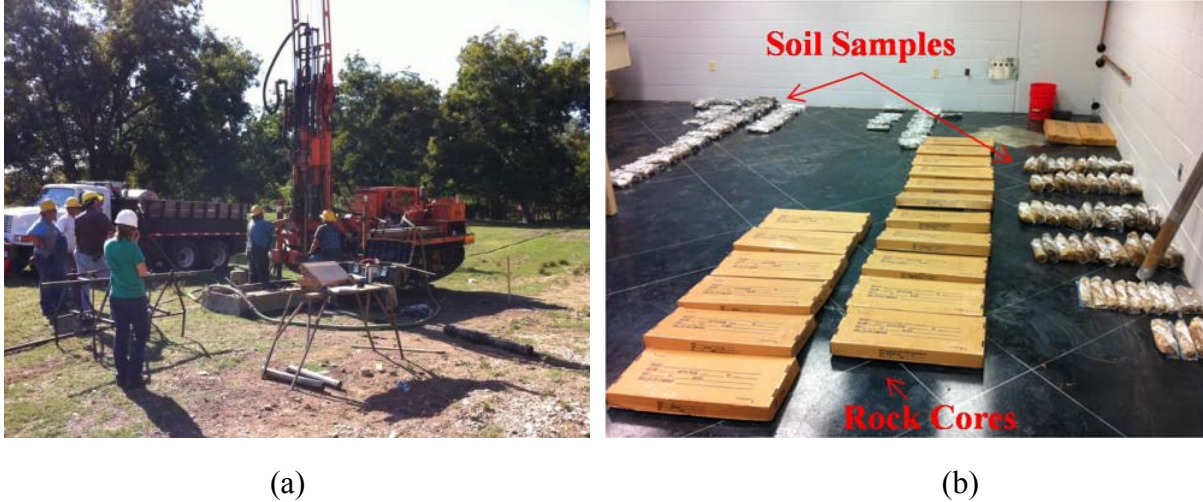
Figure 3.17. Photograph of (a) geotechnical investigations performed by UofA in conjunction with AHTD at Siloam Springs Arkansas Test Site, and (b) UofA stored rock cores and soil samples.
