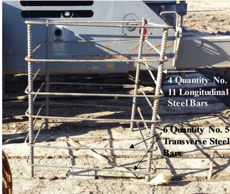
Figure 6.5. Photograph of extra reinforcement for the test shaft T-4N top block reinforcement cage.
