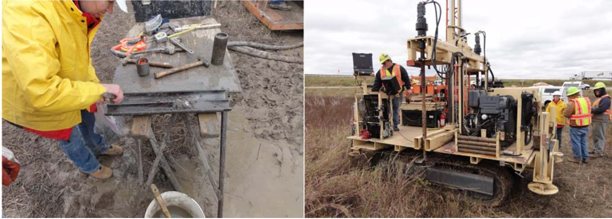
Figure 3.18. Photograph of (a) bulk sample collection performed by UofA personnel at the TATS, and (b) MODOT CPT rig.
