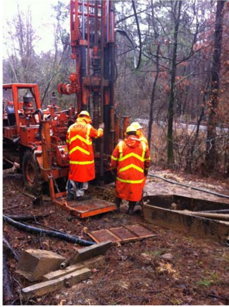
Figure 3.19. Photograph of (a) geotechnical investigations performed by UofA in conjunction with AHTD at Monticello Arkansas Test Site, and (b) UofA UU triaxial compression test sample.
