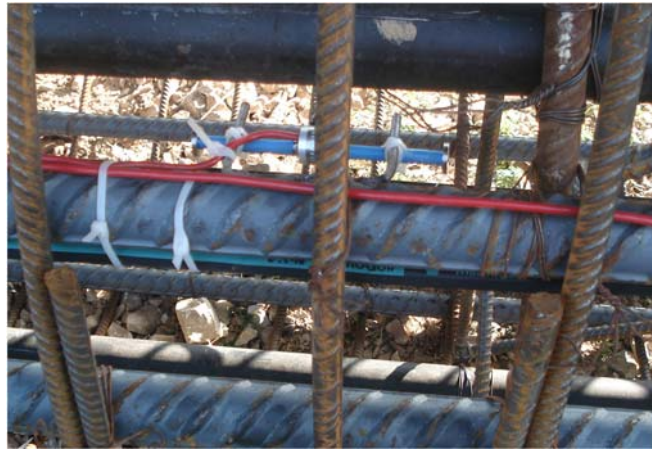
Figure 5.7. Photograph of installed vibrating wire strain gauge utilizing welded mount and zip ties.
